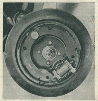
Fig. 46. Adjusting the Trojan's Brakes Adjuster cap is arrowed.
