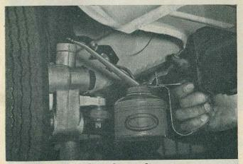
Fig. 14. ISETTA STEERING LUBRICATION
