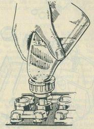
FIG. 40. TOPPING-UP BATTERY CELLS
