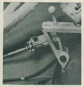
Fig. 55. Trojan Gear Control
