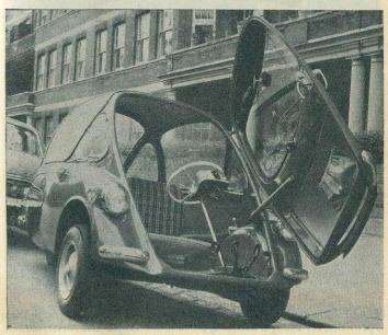
FIG. 1. FRONT OPENING DOOR OF THE TROJAN
