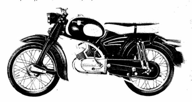
Genuine 3-speed ZUNDAPP engine, two-stroke, aluminium alloy cylinder with hard-chromium lined, wear-resistant surface, specially inclined-jet carburetter with air cleaner. Fuel: petrol-oil mixture. Ratio 20:1 for running-in. later 25:1, exhaust efficiently noise-muffling with deep sound. BOSCH-flywheel-magneto 28 watts, transmission of 3 speeds and idling, kickstarter, foot-change, oil-bath lubricated multiplate clutch.
