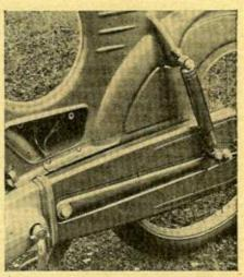
large proportion of cast light metal in the construction-the entire rear frame is formed from an alloy casting-keep noise and drumming down to a minimum.
