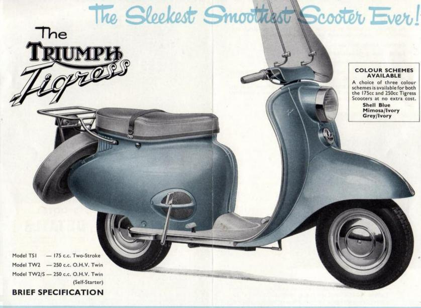
ENGINE TSI 173 c.c. single cylinder two stroke fan cooled, Flywheel magneto, Steel connecting rod with roller bearing big end, Petroil Iubrication.
