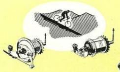
Internal expanding Sturmey-Archer front (BF) and rear (BR) brakes are world famous. This principle is combined with a 3-speed wide ratio gear in the AB.
