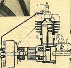
A section through the engine showing the well-supported shaft driving the roller and the "Wipac" flywheel magneto. When fitted, of course, the cylinder lies horizontal.
