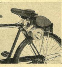
The unit presents a neat appearance when seen from the near side, on which a large domed cover enshrouds the flywheel magneto.
