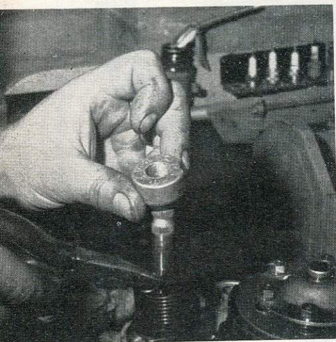
Kickstart spring retainer is held in position with a circlip. Remove this, then the retainer and spring from shaft.
