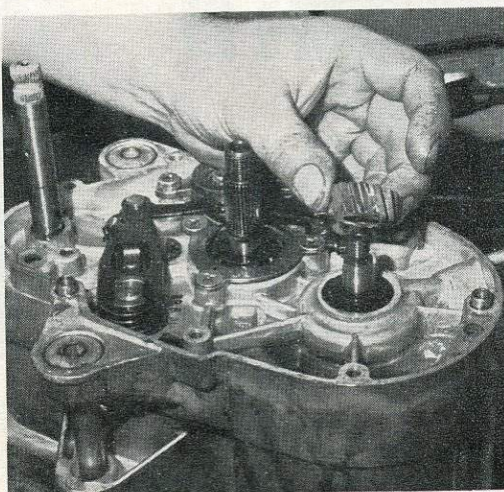
Nut holding the drive pinion on, can now be removed. Pinion is on tapered shaft and should be eased off with wedge.
