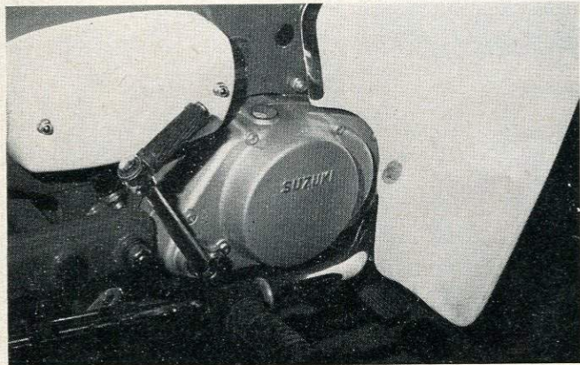
Wide, deep legshields are fitted which keep a lot of rain off driver's legs. They also keep the back half of the engine nice and clean preventing dirty clothes.
