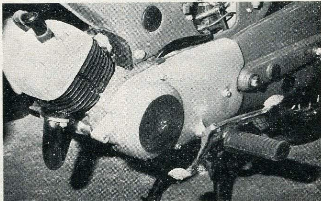
With the legshields quickly removed the engine is very accessible for normal adjustments or major work. Gearchange is rocking arm pedal.
