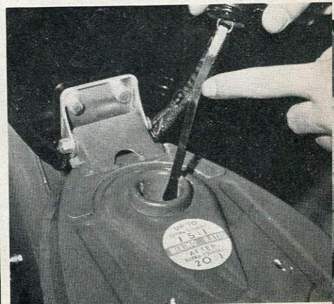
Petrol cap has a useful measure hung beneath it. At last—you can stop at a garage and know how much fuel to get.
