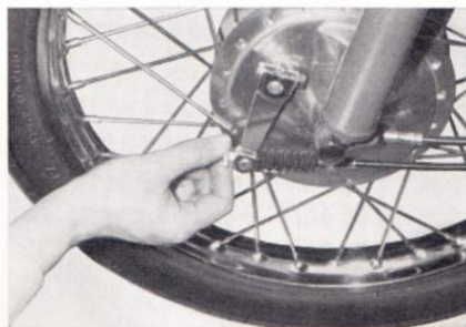
Fig. 48—Adjusting Front Brake
