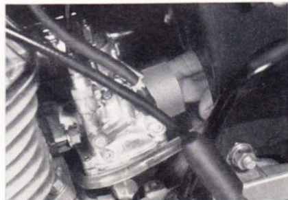
Fig. 20—Checking Throttle Valve Movement
