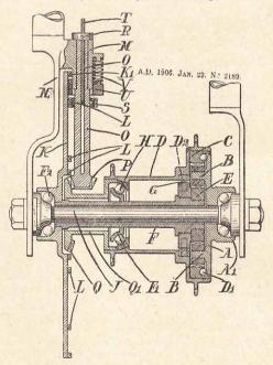
comprises a sleeve AI, on which is adapted to screw a free-wheel or the like. This sleeve has fixed to it the planet carrying pins B. The internally toothed ring C is fixed to the hub shell D, which at that end may be mounted upon ball bearings DI upon the planet pinion carrier A. The sun pinion E is fixed to a sleeve F hereinafter termed the sun pinion sleeve. Between the hub shell and this
