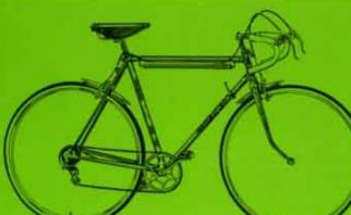
Frame: 191", 214" and 221" Wheats: 26" x 11" on 191" size 27" × 13" on 214" and 224" skin-nided Sprite tyres. Sear: Hurst Swifto Mk. II 5-speed with red rollers. landlebar: Brampton Mass alloy on Brakes: Centre-pull alloy with Sun
