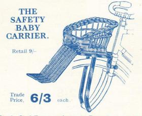
Sturdy Steel Frame to fasten to Front Fork and Hub Spindle. Enamelled Black. Wicker Basket with Leg Rest and strong Leather Strap. By removing Basket, Steel Frame is instantly available as a Parcel Carrier,
