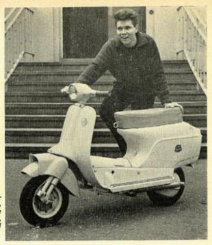
a dual saddle and automatic gearing with a claimed top speed of 35 m.p.h. will cost £87 3s. Raleigh claim that it can carry two passengers weighing 22 stone up a 1 in 9 gradient without pedal assistance. A short run two up on the demonstration model proved this fact quite acceptable.
