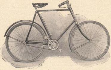
have reduced it to £15. The specification of the machine includes the patent triangulated frame with eccentric chain adjustment, Sturmey-Archer three-speed gear, A-Won clincher tyres, and Brooks' saddle. This model is made for gents as well as ladies.
