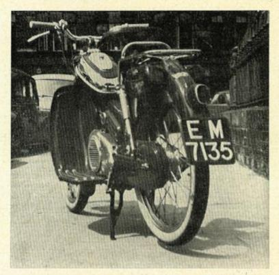
At speeds up to a little over 20 m.p.h. the power unit is very smooth and quiet but over this and up to the maximum of just under 30 m.p.h. mechanical noise and vibration become progressively noticeable. Exhaust and intake standards of silencing are very good indeed and it may be that the slight but persistent transmission whine was noticed only because the machine was otherwise better than average for quietness.
