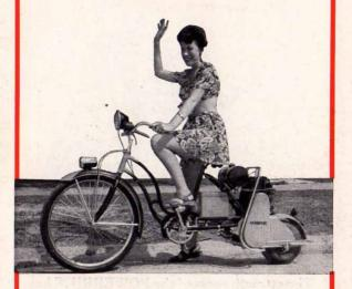
A self-contained motorized unit—quickly adaptable for use on any standard bicycle—simply by removing the rear wheel.
