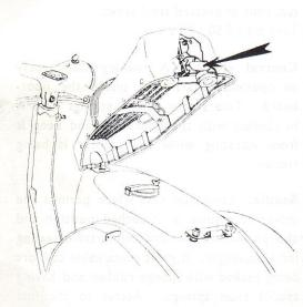
Fig. 10 - Access to the fuel tank
