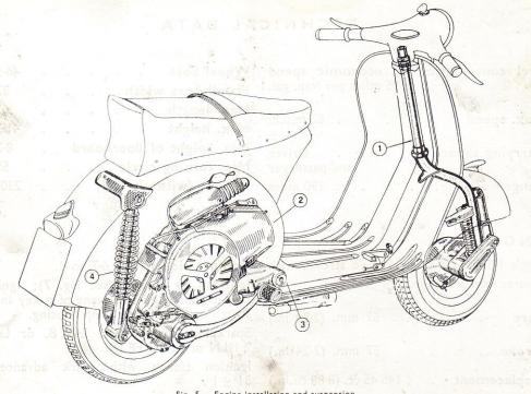
Fig. 5 - Engine installation and suspension
