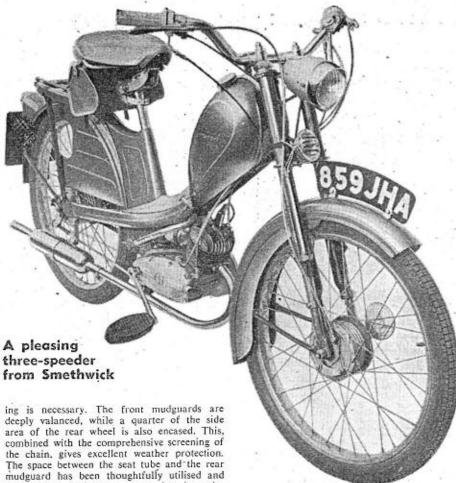
a capacious tool compartment has been installed at this point.
