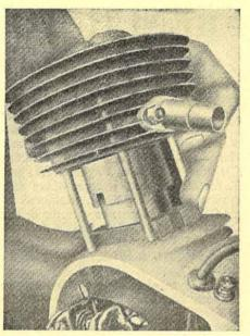
Use of a simply-made support plate ensures that the piston skirt will not suffer damage during removal and replacement of the Rex cylinder barrel. The plate should be made from a piece of clean hardwood, with no splinters or saw-dust left around the cut edges. Dimensions are given in this article.
