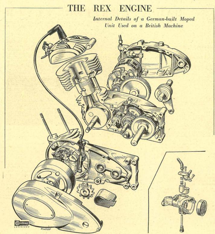
Power unit of the Phillips "Gadabout," as well as of the range of Rex mopeds, and of the projected Dunelt machine, the Rex engine is a 49-c.c. two-stroke developing 2.1 b.h.p. at 6,000 r.p.m. and running on a compression ratio of 6.8 to 1. It hails from a German factory long famous on the Continent for precision engineering.
