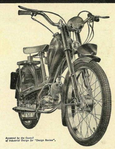
Specification includes: 49 c.c. engine with 2-speed unit construction, giving a power output of 2.1 b.h.p., Magdyno Lighting, Tubular Frame. Telescopic Forks and complete with electric Horn, Number Plates and Licence Holder.
