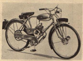
(Right) A faired and polished primary-drive cover enhances the appearance of the 49 c.c. engine in the new Phillips cyclemotor. Final drive is from a clutch and counter-shaft.
