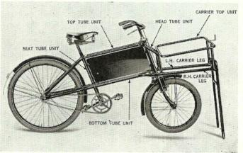
This bicycle is designed specially for easy replacement of any component in the event of damage. From an export angle an important factor is that all parts are detachable, thereby facilitating easy package. The main frame is constructed from duplex stays to give added strength. The machine is built as a light commercial vehicle, rather than a standard bicycle with a basket carrier added.
