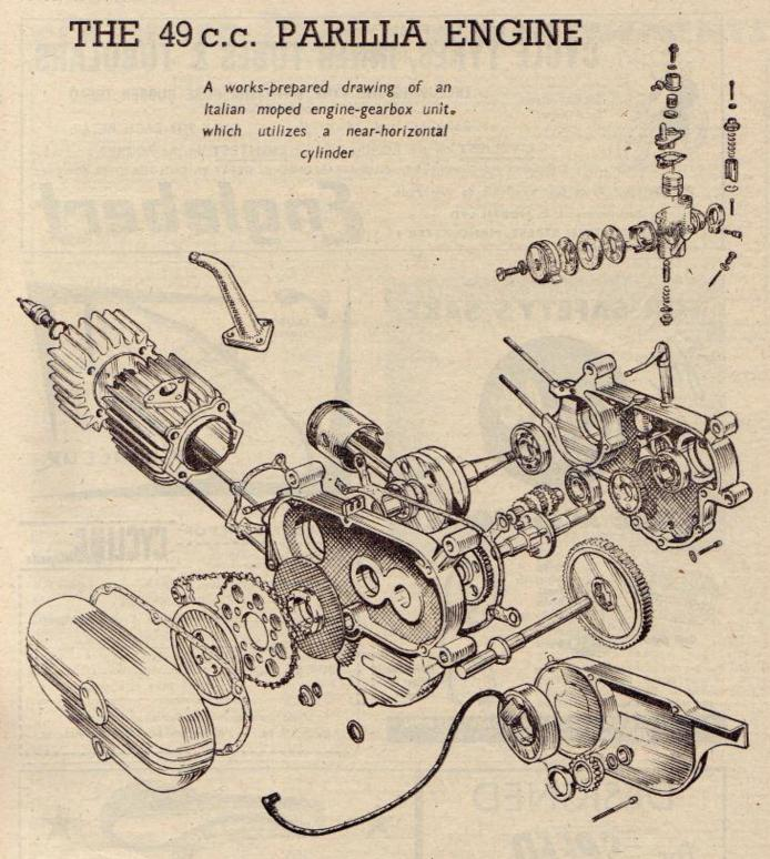
F all high-performance mopeds, the 49-c.c. Parilla is perhaps the simplest in conception. It is powered by a two-stroke engine (though there are also four-stroke variants) of the property of the stroke develop-38 m.m. bore x 44 m.m. stroke, developing 1.7 b.h.p. at 5,500 r.p.m. It is this unit which is illustrated here, in a drawing based on one issued by the Parilla factory.
