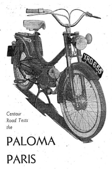
THE new Paloma Paris, an improved form of the Paloma D.A.S.L., might well be described as the ideal about town moped. Easy steering, good road holding, rapid automatic acceleration from the Lavalette engine and Multimatic progressive clutch, all make for smooth,
