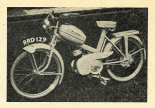
starts the engine, as the revs mount so the second stage comes in and takes over the drive up to about 8 m.p.h. when the final, solid drive stage cuts in with a light "clonk" almost as though one has changed up.
