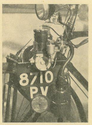
transfer port. The latter was drilled up the boss from the base, then across into the cylinder, the outside holes afterwards being plugged up.
