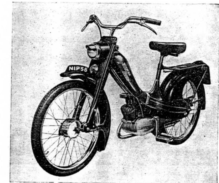
handlebar. Tyres are 23in. x 2in. and full width hub brakes are provided on both wheels.
