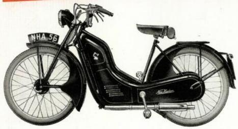
THESE SALES POINTS SPEAK FOR THEM-SELVES 98 c.c. Engine. Complete enclosure. Valanced guards for extra weather protection. Sturdily-built frame. Heavy duty tubular spring fork. Adjustable clip fixing motor-cycle type handlebar with welded control levers.
