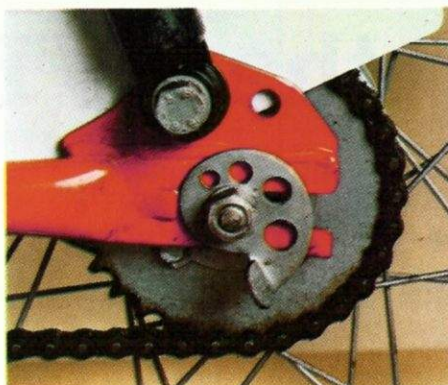
Rear chain adjustment is by snail cams, a great aid to quick and easy chain tensioning and wheel alignment
