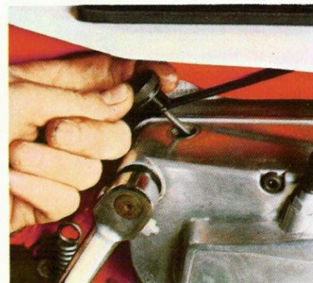
Transmission oil is checked with the dipstick on the top of the right engine case under the platform
