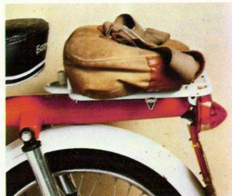
The rear rack has a spring loaded clip which is quite handy for small pieces of shopping or bags
