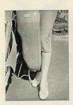
Another point to noce: the smart NSU leg shields can be fitted to any Quickly, and this transforms the moped in a moment into a vehicle offering the smartness and the protection of a scooter.
