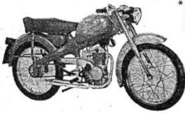
\* MOTOM '60S, net weight 1251b., maximum speed 47 m.p.h. with a fuel consumption of 226 m.p.g. The four-stroke engine is overhead valve air cooled, 51 c.c. capacity, power 2.9 h.p. and a compression ratio of 8.2: 1. Three speed mesh gear, foot gear change, kickstarter, telescopic front and rear suspension. 2½in. x 17in. tyres, drum brakes. Racing type saddle. Fuel tank 1¾ gallon capacity. Flywheel magneto-fed lighting system. Three beam headlamp, rear lamp with stop light and reflex reflector.
