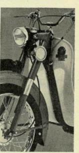
CHECK: Easily-replaced legshield; speedo as standard; sensible-size wheels for infallible roadholding.
