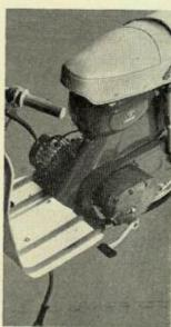
TRY OUT: Fan-cooled engine with high output at low revs; 3-speed gear box as used on 125 c.c. model; flat platform with clear legspace.
