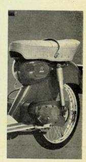
APPRECIATE: Oildamped swinging arm; full shielding round rear wheel; long broad dualseat for big man comfort.
