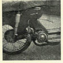
WHEELS: Tyres 16 x 2.25, expanding brakes. ELECTRICS: Flywheel/magneto, 6 volt
