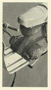
TRY OUT: Fan-cooled engine with high output at low revs; 3-speed gear box as used on 125 c.c. model; flat platform with clear legspace.
