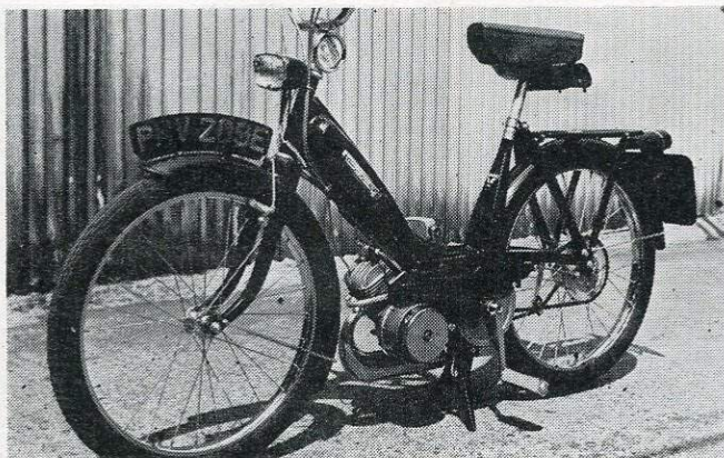
The 'Cady' is far less like a motorcycle too look at than the Sports 50 and performs like a moped. Top speed is around 25 mph on a flat road.
