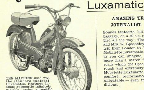
clude automatic infinitely variable gearing, automatic di-moby clutch, high efficiency 49 c.c. engine, with chrome lined cylinder and flat top piston, developing 2.8 h.p. at 5,500 r.p.m. Pressed steel frame, new design suspension, built for trouble free riding on the roughest roads. Finished in quality enamel and heavy chrome plating, the Mobylette Luxamatic is the machine to rely on—especially when the going gets tough.
