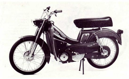
Specifications: Engine: 49.9cc. Two Stroke. Compression Ratio: 8.6: 1. 2.5 BHP at 5200 R.P.M. Carburettor: Gurtner. Magneto: Novi. Clutch: Automatic Dimoby with
