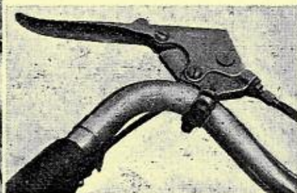
The lever, on the handlebar of the machine, which controls the engagement of the drive. It can be locked in the "on" position.
