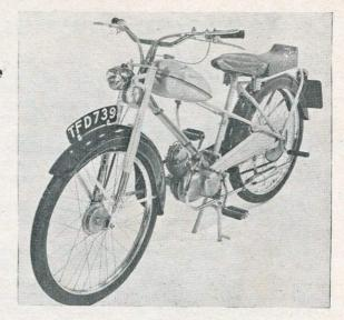
give a maximum of 2 b.h.p. at 5,200 r.p.m. which is well above the average for current mo-ped power plants. The novelty of the fourstroke engine has the added interest of a performance on the road that is quite unusual, speed, acceleration and revs all being well over the figures for most similar sized two-strokes. A mean maximum of 36 m.p.h. in top gear was recorded and this speed was reached without any waiting for it, while the low gear getaway was a constant surprise.
