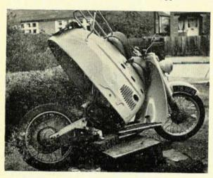
For a quick look at the engine, the body shell is tilted forward. If the hinge bolt is removed, the shell itself will come right off
