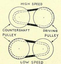
shaft pulley sides being forced apart by the pressure of the belt.
