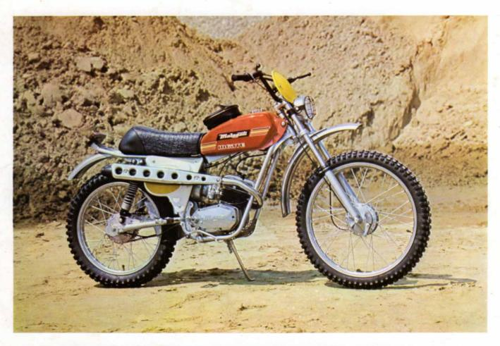
Frame is duplex type with reinforcement at stress points and fitted with Marzocci hydraulic front forks. Rear suspension by swinging arm hydraulically damped by units with three position ride control. Standard equipment includes crankcase shield, headlamp stone guard, tank pouch and ball ended levers with gaiters.
