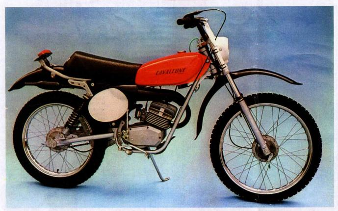
Frame is duplex type with reinforcement at stress points and fitted with Marzocci hydraulic front forks. Rear suspension is a semi-cantilever design permitting long travel and controlled by adjustable hydraulic units. Standard equipment includes kick start, crankcase shield, handlebar map-bag and ball ended levers with gaiters.
