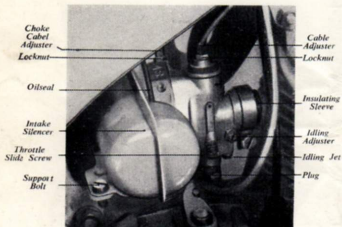
ILLUSTRATION 6 R.50: Carburettor, right hand, with Air Intake Silencer.
