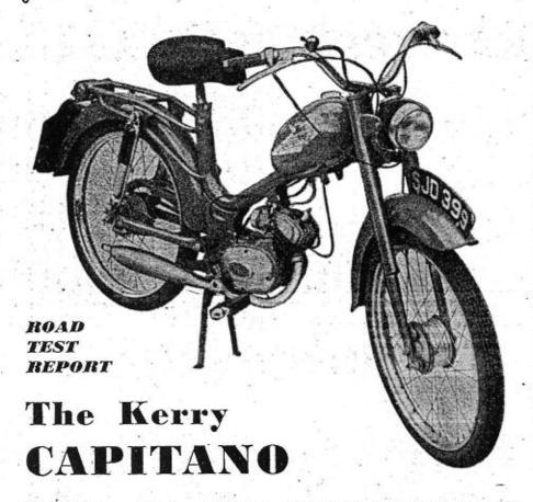
MATCHED in a contest of speed with most other standard production mopeds as distinct from the high performance sports machines, the Kerry Capitano would probably be unchallenged. For the compact 47.6c.c. engine, developing 1.8 b.h.p. at 5,000 r.p.m., is a real little powerhouse with a seemingly inexhaustible reserve of drive.
