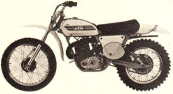
KTM 125, 250 & 400 MOTO-CROSS MACHINES. New type Ceriana forks with 198 mm travel. New lightweight frame and swinging arms. Shoulderless Akront rims. Improved engine performance.
