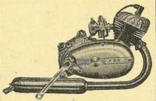
"The silent Mo-Ped Engine", built by one of the oldest Italian Makers, MORINI & MINARELLI of Bologna. Two-speed & 3-speed 48.c. models. Pedal kick start from rest, back pedalling rear brake actuation. Low petrol consumption. powerful yet silent. Also 75 c.c. models, two-stroke, 3-speed with kick start.
