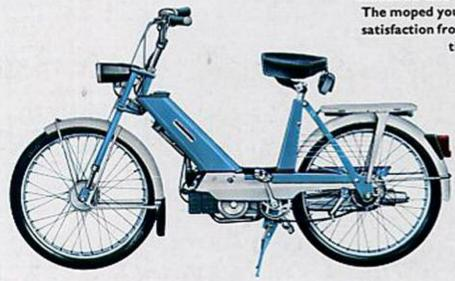
The Jawa — Babetta • two stroke, air cooled single cylinder of 50 c. c. swept volume • serves as an ideal lightweight means of transport for city traffic, short trips, and holidays • This simple and most serviceable moped has been designed with due regard to riding comfort and easy maintenance
