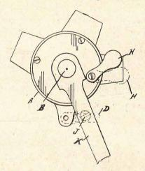
of the ratchet, thereby allowing the machine to be wheeled backward without putting on the brake. A small spring-controlled projection J is formed upon the pedal crank K, which projection passes over the lever arm during back-pedalling, but immediately the pedals are reversed for the drive, the spring projection J presses the lever arm H into its normal position, and allows the machine to be driven forward, thus automatically bringing brake mechanism into action.
