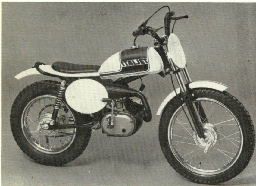
Trials version of the Junior Cross, with automatic gearbox.
