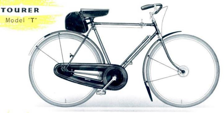
FRAME: 19", 21" and 23". Double tapered seatstays. Built of special quality parallel steel tubing. Entirely brazed-up. Specially cut-away lugs. Brazed-on pump pegs and reflector eye. FRONT FORK: "D" to round fork blades. Narrow pattern crown. Solid ends. WHEELS: 26"×1½" Dunlop Endrick rims. TYRES: Dunlop Roadster. GEAR: 3-Speed hub. GEARCASE: Hercules detachable oilbath. HANDLE-BAR: "Comfort Pattern" raised, celluloid covered on adjustable clip. Rubber grips. BRAKES:
