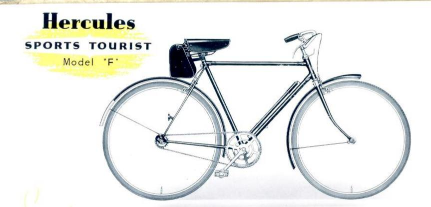
FRAME: 19°, 21° and 23°, double tapered seatstays. Entirely brazed-up. Cut-away lugs. Low built. Short wheelbase. Brazed-on pump pegs and reflector eye. WHEELS: 26°×12° Endrick steel. TYRES: Dunlop Sports. HANDLEBAR: 18° "Comfort Pattern" raised. BRAKES: Hercules front and rear caliper. MUDGUARDS: Hercules narrow steel. SADDLE: Double texture spring seat. PEDALS: 4° rubber.
