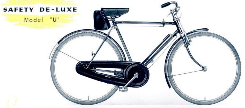
FRAME: 19", 21" and 23", double tapered seatstays. Low built with short wheelbase. Entirely brazed-up, Cut-away lugs. Brazed-on pump pegs and reflector eye. WHEELS: 26" × 13". TYRES: Dunlop Roadster, GEAR: 3-Speed, top tube control. CRANKS: 6½". GEARCASE: Hercules detachable oilbath. HANDLE-BAR: "North Road" high raised with roller levers. Rubber grips. BRAKES: Front and rear rim.
