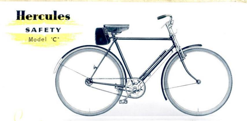
FRAME: 19°, 21" and 23°, double tapered seatstays. Specially low built. Short wheelbase. Entirely brazed-up. Cut-away lugs. Brazed-on pump pegs and reflector eye. WHEELS: 26" × 13". TYRES: Dunlop Sports. HANDLEBAR: "North Road" high raised with roller levers. Rubber grips. BRAKES: Front and rear rim. SADDLE: Double texture spring seat. PEDALS: Rubber. FITTINGS: Reflector, inflator,
