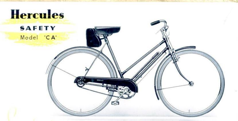
FRAME: 19", 21" and 23", double tapered seatstays. Low built bracket. Brazed-up seat and chain stays. Cut-away lugs. Brazed-on pump pegs and reflector eye. Short wheelbase. WHEELS: 26" × 18". TYRES: Dunlop Sports. CHAINGUARD: Metal. HANDLE-BAR: "North Road" high raised with roller levers. Rubber grips. BRAKES: Front and rear rim. SADDLE: Double texture spring seat. PEDALS:
