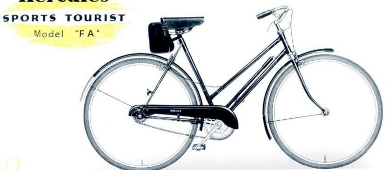
FRAME: 19", 21" and 23", double tapered seatstays. Entirely brazed-up. Low built. Short wheelbase. Brazed-on pump pegs and reflector eye. WHEELS: 26"×13" Endrick steel. TYRES: Dunlop Sports. HANDLEBAR: 18" "Comfort Pattern" raised, BRAKES: Hercules front and rear caliper. CHAINGUARD: Metal. MUDGUARDS: Hercules narrow steel. SADDLE: Double texture spring seat,
