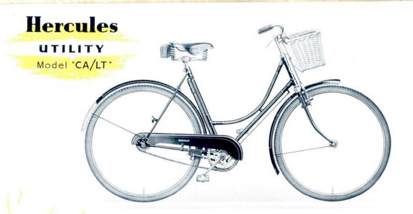
FRAME: 19", 21" and 23". Built with loop tube. Double tapered seatstays. Low bracket. Brazed-on seat and chain stays. Cut-away lugs. Brazed-on reflector eye. Short wheelbase. WHEELS: 26" × 13". TYRES: Dunlop Sports. CHAINGUARD: Metal. HANDLEBAR: "North Road" high raised with roller levers. Rubber grips. BRAKES: Front and rear rim. SADDLE: Leather 3-coil. PEDALS:
