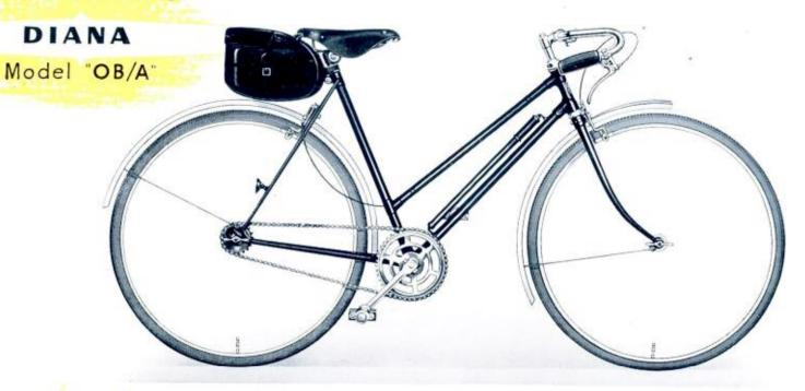
FRAME: 19", 21" and 23". Double tapered seatstays. Entirely brazed-up. Specially cut-away lugs. Low bracket. Short wheelbase. Brazed-on pump pegs and reflector eye. WHEELS: 26"×1½" Endrick steel. TYRES: Dunlop Sports. HANDLEBAR: Racing pattern, chromium plated, on adjustable stem. Rubber grips. Optional: Celluloid covered. BRAKES: Hercules front and rear caliper. MUDGUARDS: Hercules narrow steel, white enamelled. SADDLE: Leather racing. PEDALS: Rubber. FITTINGS:
