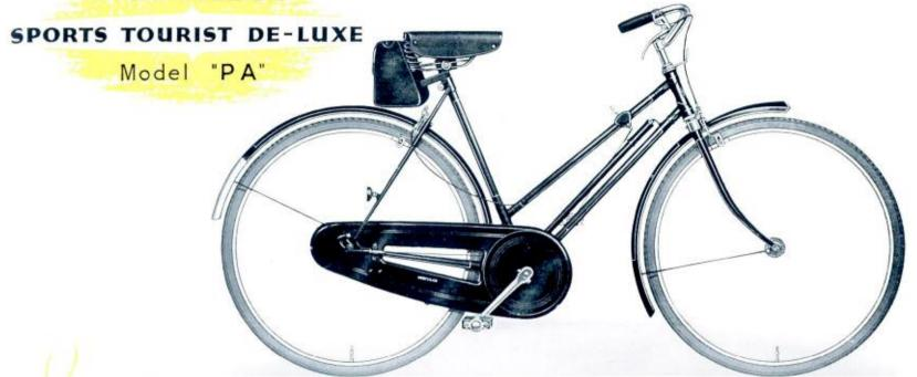
FRAME: 19", 21" and 23", double tapered seatstays. Entirely brazed-up. Low built. Brazed-on pump pegs and reflector eye. Short wheelbase. WHEELS: 26"×1\frac{1}{2}" Endrick steel. TYRES: Dunlop Roadster. GEAR: 3-Speed, top tube control. 44T chainwheel, 6\frac{1}{2}" cranks, 18T sprocket. GEARCASE: Hercules detachable oilbath. HANDLEBAR: 18" "Comfort Pattern" raised. BRAKES: Hercules front and rear
