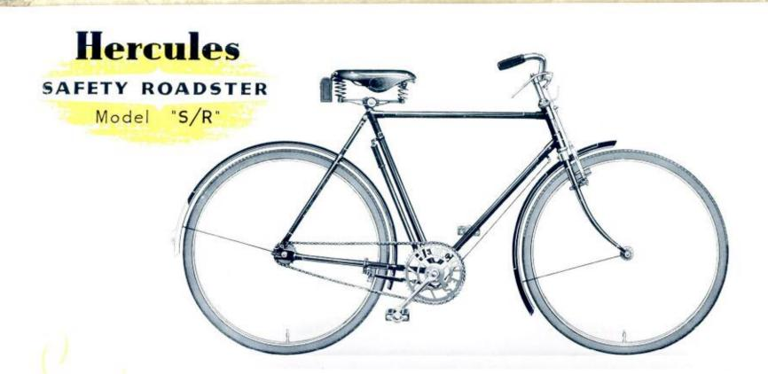
FRAME: 20", 22" and 24", low bottom bracket. 10½" ground clearance. WHEELS: 26" × 1¾" Westwood steel rims. Hercules chromium plated. SPOKES: Rustless. TYRES: Dunlop. GEAR: 69". HANDLE-BAR: "North Road" raised with roller levers. BRAKES: Front and rear rim. SADDLE: 3-coil leather. PEDALS: Rubber. FITTINGS: Tools,
