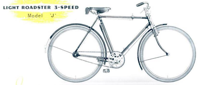
FRAME: 22°, 24° and 26°, sloping top tube. WHEELS: 26°×13°. TYRES: Dunlop. GEAR: 3-speed hub. HANDLEBAR: "North Road" high raised. Optional: "North Road" dropped. BRAKES: Front and rear rim. SADDLE: Leather 4-wire. PEDALS: Rubber. FITTINGS: Toolbag, tools, inflator and reflector.
