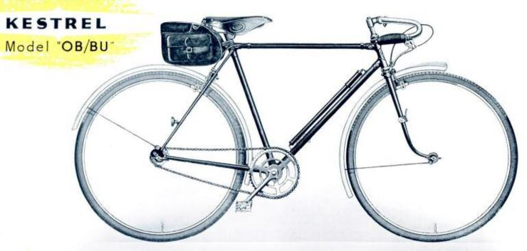
FRAME: 21" and 23" upright. Double tapered seatstays. FRONT FORK: Solid brazed-in fork tips. Russ pattern. Brazed-on detachable lamp bracket. WHEELS: 26"×1½" Endrick steel. TYRES: Dunlop Sports. HUBS: Hercules quick release with freewheel and fixed cog. HANDLEBAR: Racing pattern on adjustable stem. Chromium plated. Rubber grips. Celluloid covered optional. BRAKES: Hercules front and rear caliper. SADDLE: Leather racing. MUD-GUARDS: Hercules narrow steel, white enamelled.
