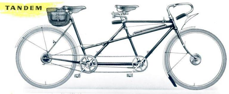
FRAME: 20½\* front, 20½\* rear; short wheelbase. Entirely brazed-up. WHEELS: Endrick tandem, 26"×1½". GEAR: Tandem 3-speed hub. BRAKES: Internal expanding hub front and rear TYRES: Dunlop Tandem 26"×1½". HANDLEBARS: Front: Highgate shallow bend, chromium plated, on swan neck stem, adjustable; Rear: Lauterwasser bend, chromium plated, adjustable. Black rubber grips.
